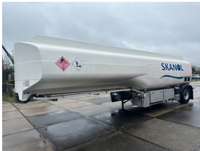
HMK BILCON 1 AXLE - 5 COMPARTIMENTEN - ADR 26.600L
