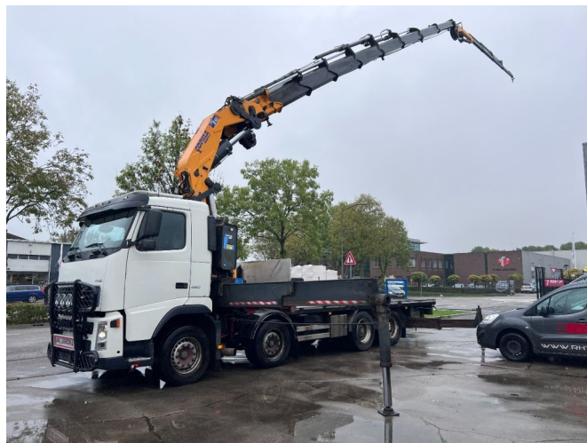
Volvo FH 12.460 8X2 + COPMA 810.8 + FLY JIB
