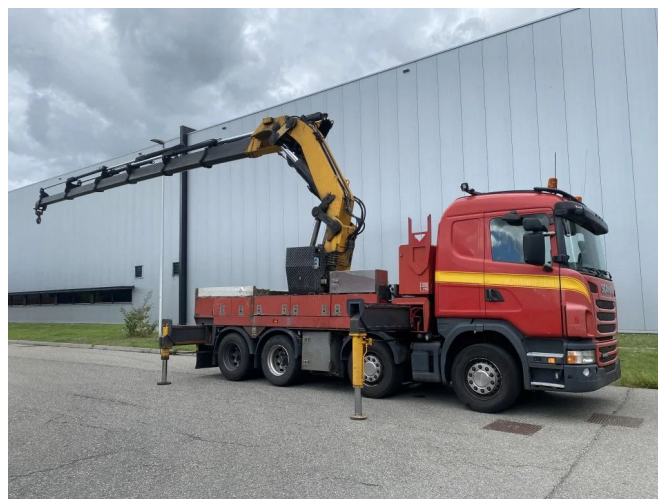
Scania G480 8X4 + EFFER 1250 6S + REMOTE + WINCH - ...
