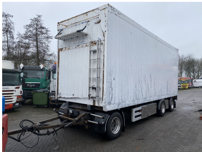
Bygg 3 AXLES - BPW + LIFTING AXLE + BOX 7,80 METER
