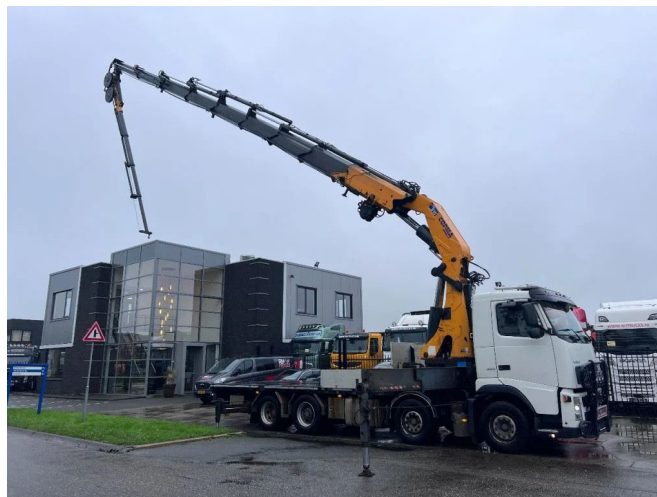
Volvo FH 12.460 8X2 + COPMA 810.8 + FLY JIB
