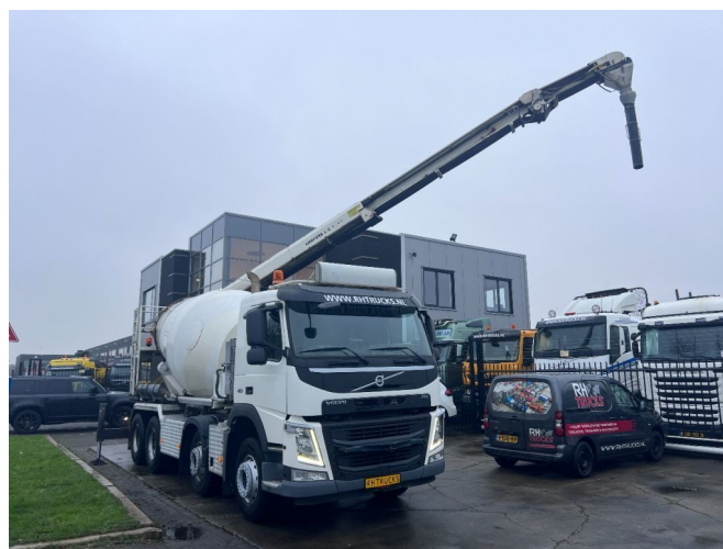
Volvo FM 410 8X4 MIXER 9m3 + LIEBHERR CONVEYOR BELT
