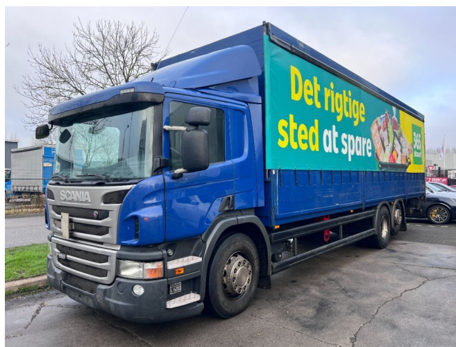
Scania P250 6X2 E6 BOX 960x248x262 + LIFT
