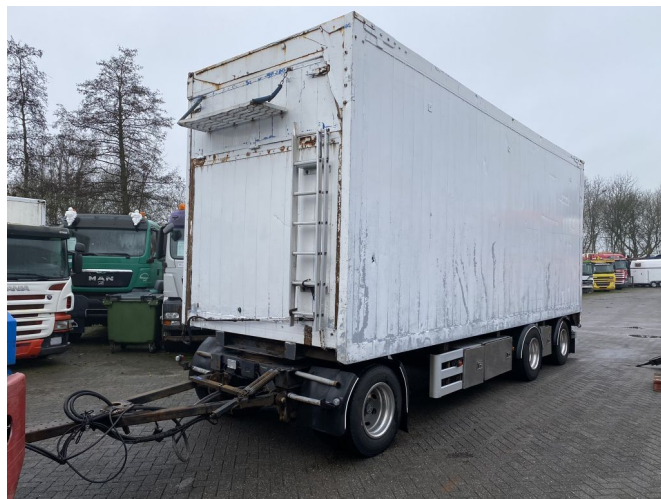
Bygg 3 AXLES - BPW + LIFTING AXLE + BOX 7,80 METER
