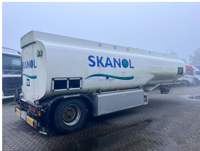
HMK BILCON 1 AXLE - ADR 26.600L - 5 COMPARTIMENTEN
