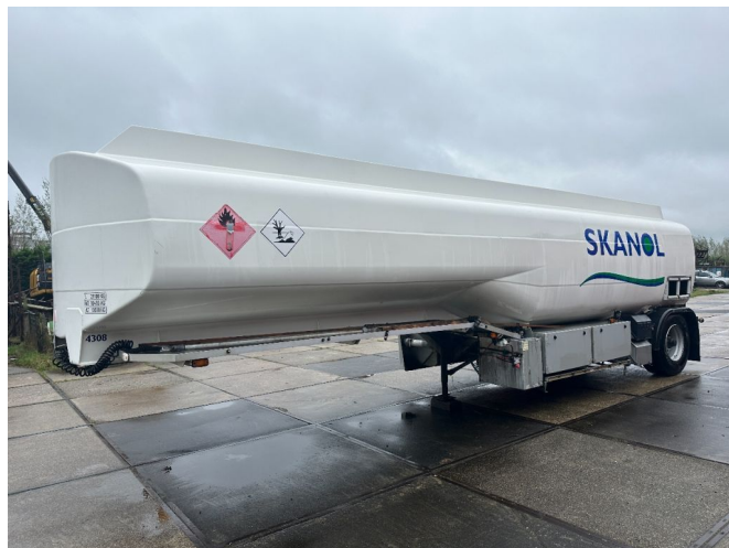
HMK BILCON 1 AXLE - 5 COMPARTIMENTEN - ADR 26.600L
